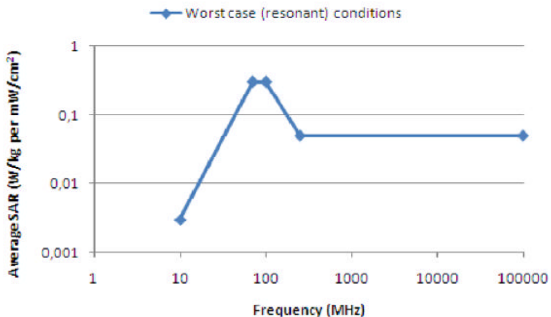
Figure 13. Radiation absorption by the human body vs. frequency, [8].
